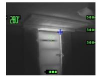
See the Heat Hot-spot tracker can be used during overhaul to locate hot spots within the structure.
